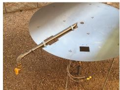
Step 5: Connect the Pilot Burner Flame Extender gas line from the appropriate gas fitting on the Ignition Control Box (see illustration page 6 of this manual) to the flare fitting on the Pilot Burner Flame Extender. Both of these fittings are flare fittings so NO pipe dope or teflon tape is needed.
