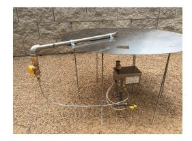
Step 6: Measure the distance between the Flat Burner Pan and the outlet of the Ignition Control Box. Install a pipe nipple with coupling in the outlet of the Ignition Control Box.
