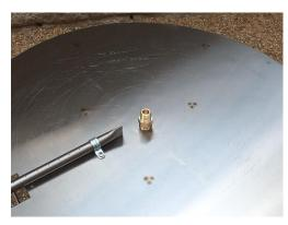
Step 8: Install the Primary Pilot Burner by hanging it on the Pilot Burner Flame Extender (as shown in photo at right) and connecting both the gas and electric to the Ignition Control Box. The Primary Pilot Burner Gas and Electrical Connections are shown in the illustration on the bottom of page 6 of this manual.
