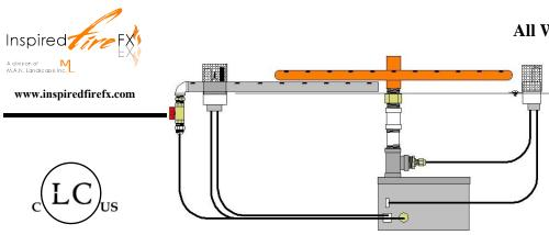
Commercial Grade All Weather Electronic Ignition System (Lateral Offset)
